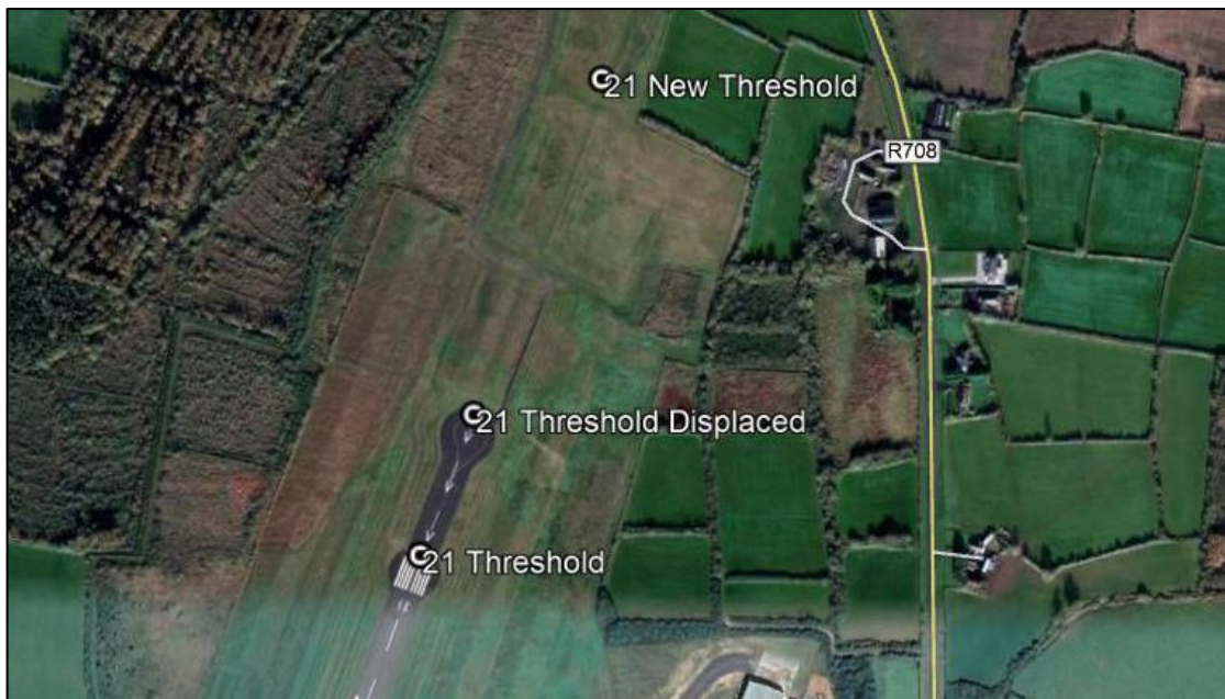
Figure 3 Runway 21 existing and proposed threshold co-ordinates
